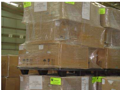
Examples of plastic pallets with feet base
